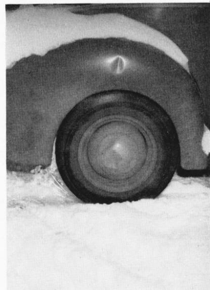
Take it easy there, mister. That's a dandy way to burn up those tires. Better put on some chains or spread some sand. Spinning won't help you out; it'll just wreck the tire.
